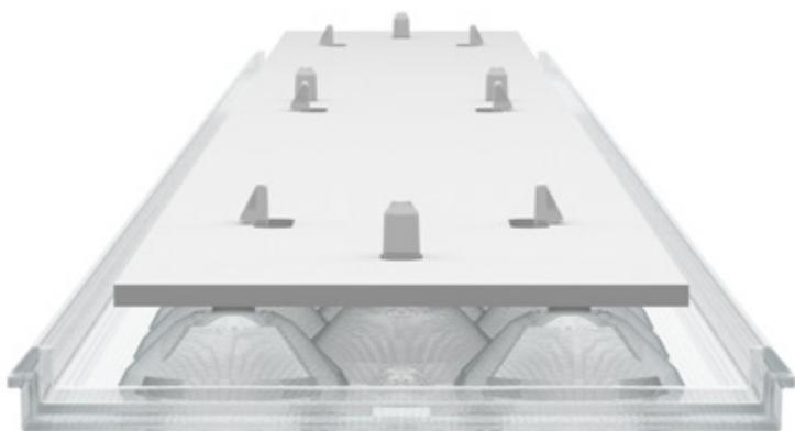
Clean, sealed, sustainable, patent-pending: LINEDO lens optics are connected reversibly with the LED boards and fit perfectly without any further sealing. They can be connected to the neighbouring lens, to the LINEDO plug or to a blank cover.
