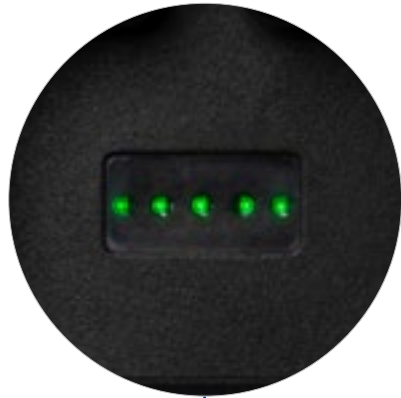
Charge level indicator
